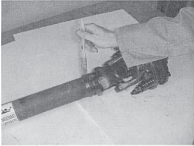
Figure 17) Grease the shield bearing grooves on the yokes and the inner telescoping member before assembly.
